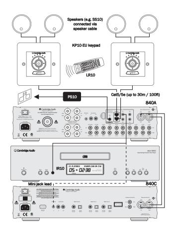
It is then possible to control the source equipment from the remote rooms by using the source equipment's own remote controls or through a learning remote. The Incognito LR10 can fully control the keypads, "learn" the source's remote control codes (including those from other manufacturers) and change source input on the amplifier etc.
